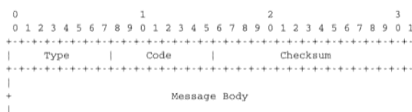
Figure 5.42: ICMP version 6 packet format
