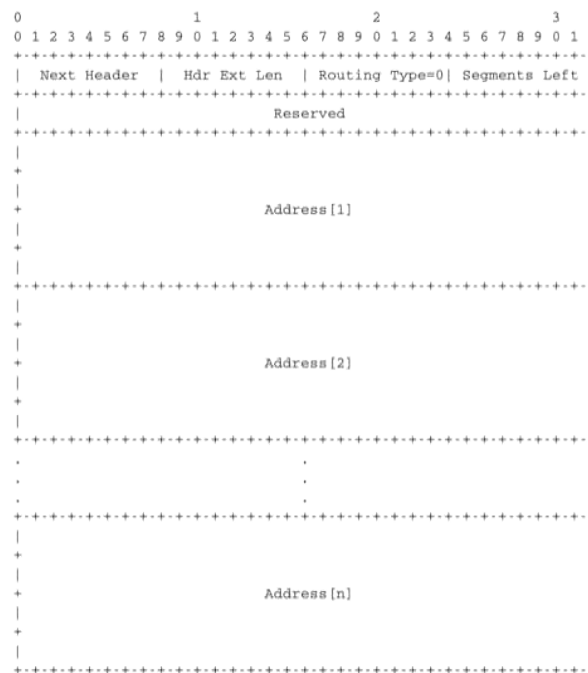
Figure 5.40: The Type 0 routing header ( RFC 2460 )
