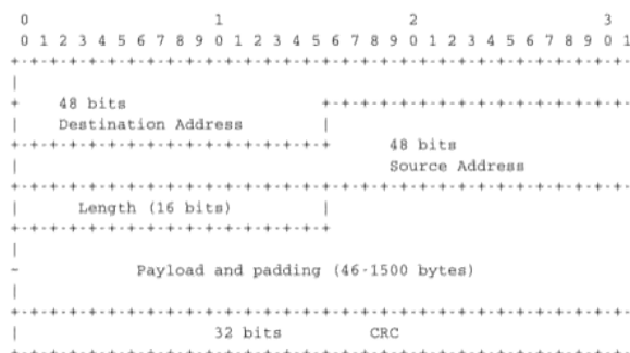
Figure 6.21: Ethernet 802.3 frame format
