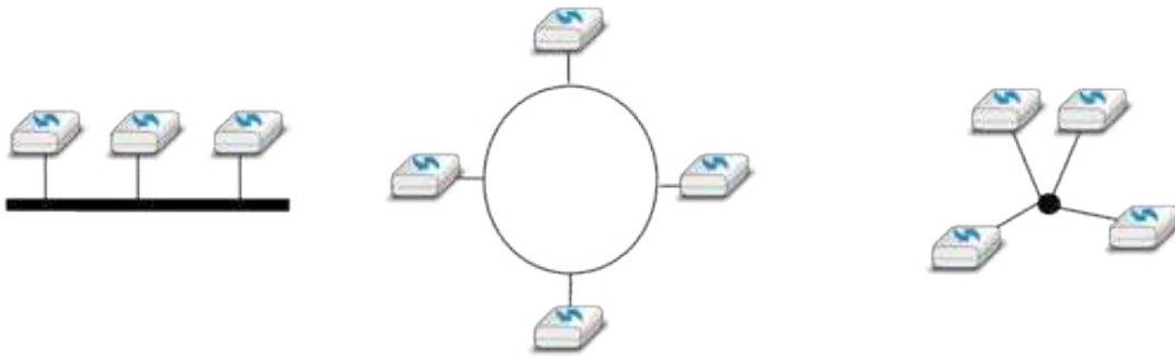
Figure 6.3: Bus, ring and star-shaped Local Area Network
